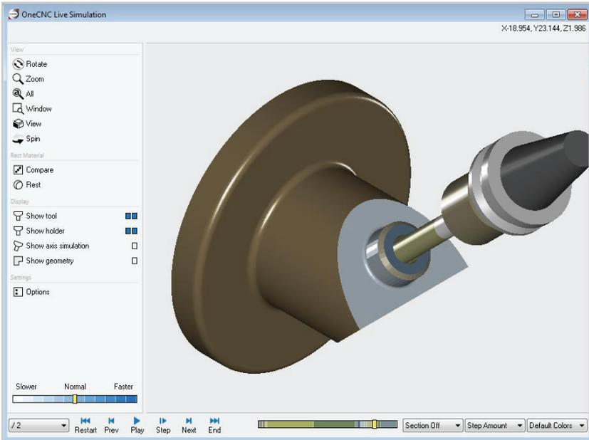
Simulate Toolpath Group #1 to see how the toolpaths are carried out, with the part rotating between plane positions.
