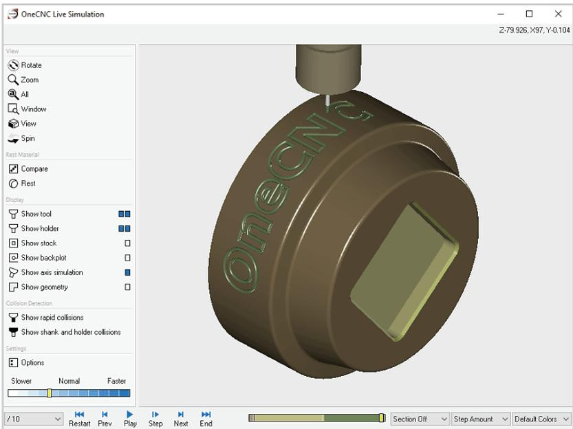
You will see how the toolpath has wrapped the vectorized text geometry around the cylinder.
