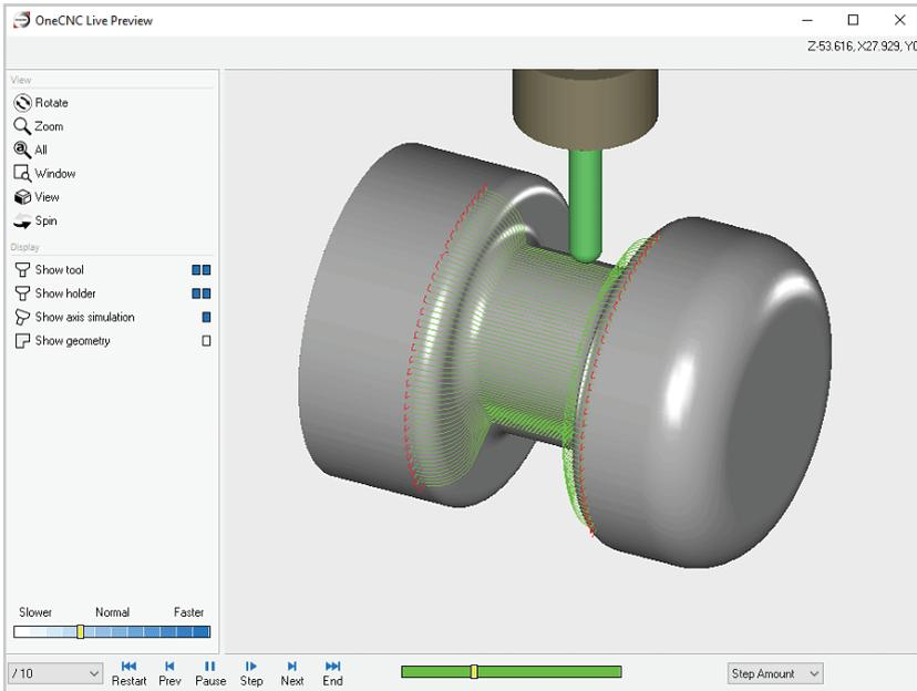
Because we selected Zigzag Toolpath the tool runs backward and forward over the part.
