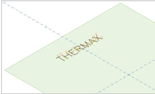
The text is engraved on the rim using a C Axis Wrap operation defined with vectorized text on the XY plane.
