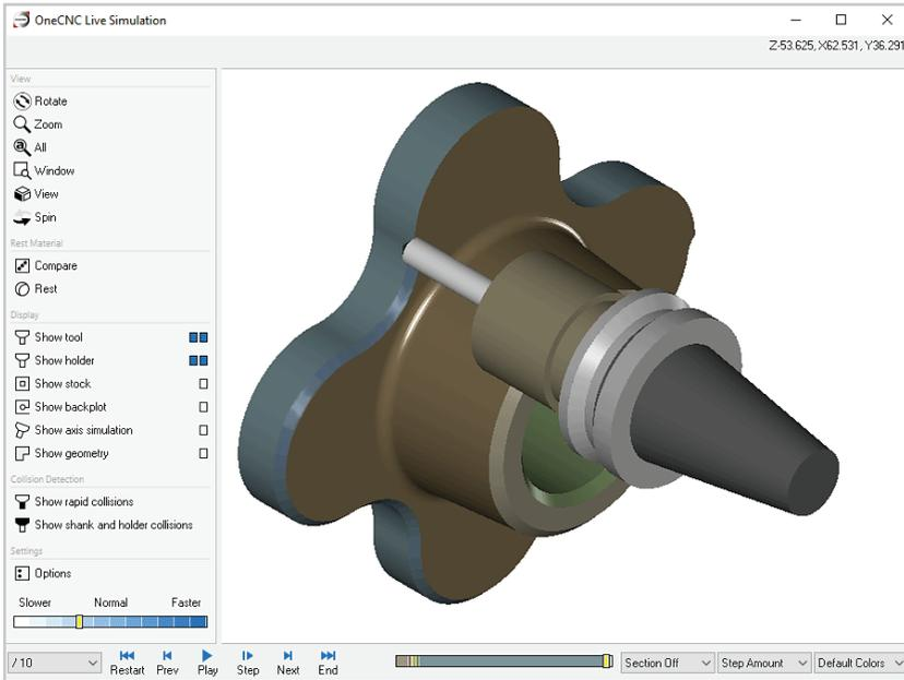
You will see the Lathe operations machine the basic shape of the part, followed by the C axis mill operations we will be working on.
