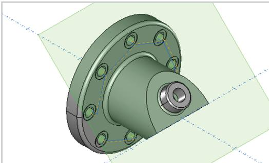
C Axis Face operations are used to drill and spot face the flange.
