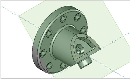
The next operation, named 7:Drill pocket face holes, drills the 4mm diameter holes in the face around the pocket.
