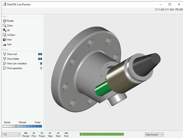
A preview of the toolpath shows it is safe to use plunge entry in this case because the open high speed pocketing strategy always plunges the tool outside the pocket boundary.
