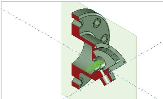
This image shows a section of the model on the XZ plane, with a backplot of the next operation which is named 6:C-Bore pocket holes.
