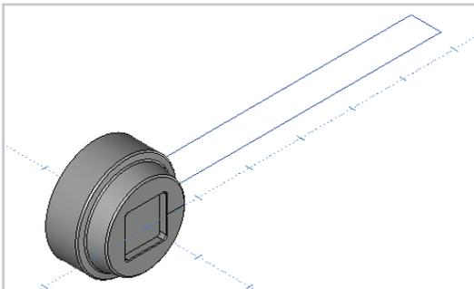
A rectangle which corresponds to the unwrapped cylinder will be drawn. The right end of the rectangle corresponds to 0 degrees and the left end corresponds to 360 degrees on the C axis.
