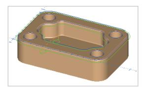
Click Finished, and the Chamfer toolpath will be created.
