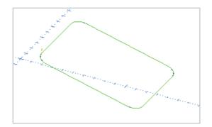
Click Finished to create the toolpath. The toolpath appears as a Cut Chain 3D operation in the NC Manager, and will preview in the drawing window when the operation is selected.
