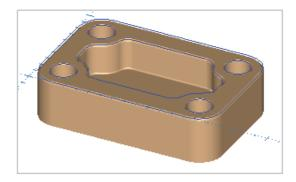
Turn off the Extracted edges layer, and turn on the Geometry and Model layers. You will see the basic outlines the part has been constructed from. These outlines are in fact all the geometry we need now to create toolpaths for the complete job.
