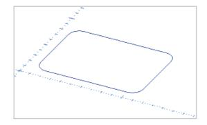
Draw a rectangle 100 x 75 with a corner radius of 10, starting at X10 Y10.
