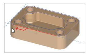
Select the outside profile as before. Set the direction as shown and press F3 to automatically select the complete profile.
