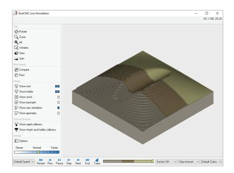
This view shows the stages of machining for the sample we will use. The first operation, seen here at the front of the view, is Z Level Roughing which has left steps on the stock. At the back of the view the Planar finish strategy has been applied.
