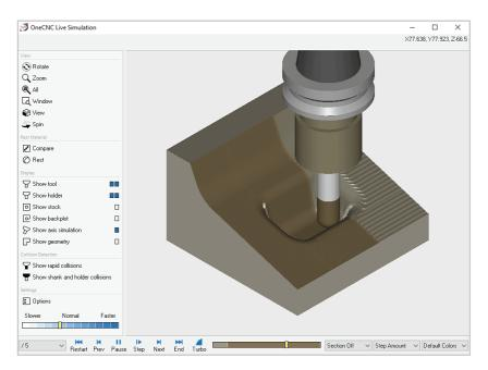
Model toolpaths are usually defined in two stages, roughing to remove the bulk of the material, and then a finishing method to cut the surface itself. For some models a semi-finish operation, which uses a finish strategy with coarser settings than usual, will be useful.
