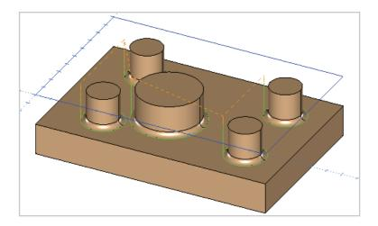
The strategy will generate a single pass to finish any fillets with a radius equal to or smaller than the tool.
