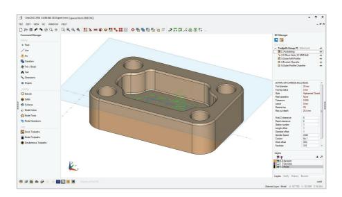
OneCNC Mill is a hybrid CAD-CAM system with a user-friendly interface. OneCNC Mill simplifies the process of defining toolpaths for the machining of parts using CNC milling machines with up to 5 axes.
