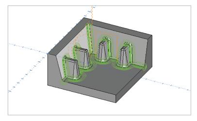
The strategy will generate multiple passes to finish any fillets with a radius equal to or smaller than the tool.
