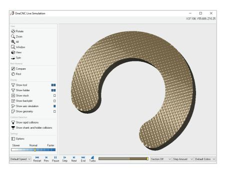
To machine the surface, draw the 2D geometry you want the toolpath to follow on a separate layer so it can be selected easily. The geometry can be drawn manually, or generated by a hatch pattern or backplot of any 2D operation.
