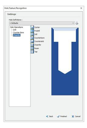
Before clicking Finished to create the hole feature toolpaths, we will save the Hole Operations list for future use as a Hole Definition. Once saved, drilling and machining for a particular bolt or hole size can be quickly applied in a new part.
