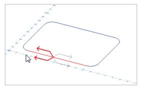
Click on the chain where you want the cut to start. Click as shown to set the direction of travel, it doesn't matter which side of the chain you select as the toolpath is not offset.
