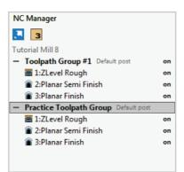
Right click on the Planar Semi Finish operation in the duplicated group and delete it using the Delete Operation command on the context menu.
