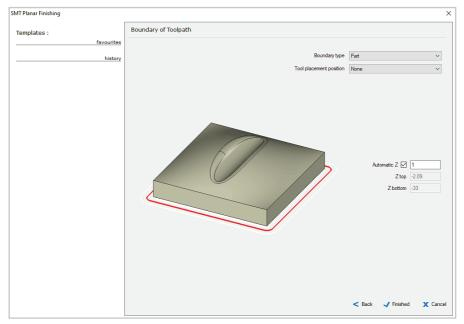
In the Boundary of Toolpath dialog, select the Part boundary option. Select None for tool placement, which allows the cutter centerline to travel up to the boundary.
