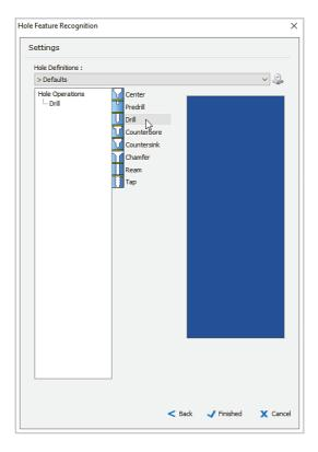
Click on the Drill icon and a new drill operation will be added to the Hole Operations list.
