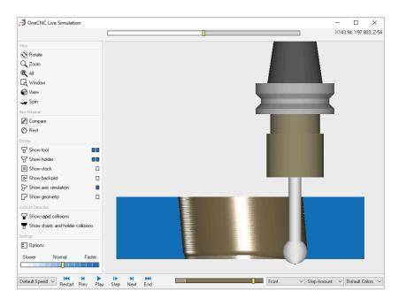
OneCNC prevents the shaft from contacting the part, so the amount of undercut possible is determined by the tool size.
