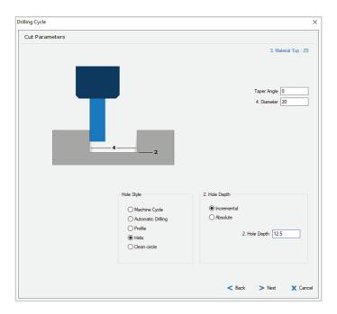
Select the Helix Hole Style option, which creates the hole by machining down a helical ramp.
