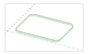
Click Finished to create the toolpath. The toolpath appears as a Cut Chain 2d operation in the NC Manager, and will preview in the drawing window when the operation is selected.
