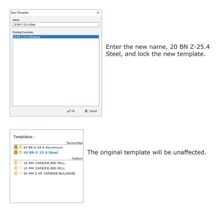
You now have two pocketing templates which can be applied quickly and easily.
