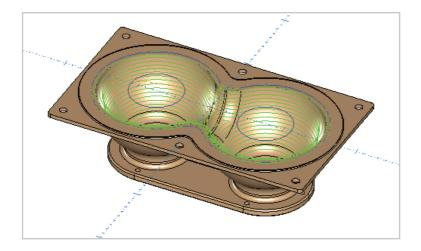
Because the boundary controls the flow of the tool path it is possible to create a good machining flow over part shapes which are otherwise difficult to machine.
