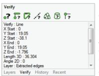
By clicking on various lines, and reading the sizes in the Verify panel, you will soon see we are dealing with a part designed in inch measurements.
