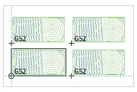
Like the multiple offsets method, OneCNC writes each of the toolpath operations as a separate subroutine in one NC file. Each subroutine will run at each offset location, which will be written to the G52 work offset. This method can be backplotted or simulated.
