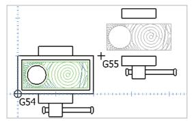
Each subroutine will be run at each location, by writing the work offset G code (G54, G55 etc) for each location before each subroutine call. As the offset positions are set on the machine and not in OneCNC, the machine operator must set the offsets correctly, and this method cannot be backplotted or simulated.
