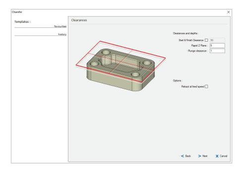
In the Clearances dialog, the only entries required are those for Rapid Z Plane, which we will set to 5, and Plunge clearance, which we will set to 1.
