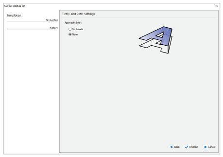
The Path Creation settings allows you to mill to the full depth in more than one pass, but for this example select None for the Toolpath style.
