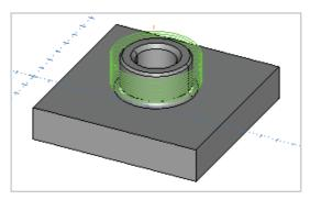
Thread Milling is an efficient means of cutting a thread, especially for larger diameters. With a single tip the toolpath follows a helical path corresponding to the pitch of the thread.
