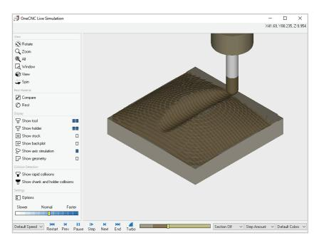
Simulate the toolpath group and you will see the semi finish operation after the initial roughing is complete.
