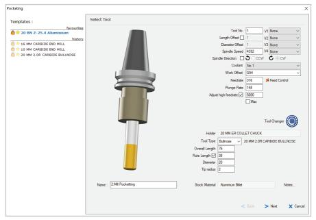
Double-click on the template you just saved and all the dialogs of the toolpath wizard will be pre-loaded with the template settings. Step through the dialogs of the wizard without changing any settings, and click Finished.
