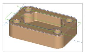
The new toolpath is created, and an instant preview will be displayed in the drawing window. The Facing toolpath operation appears under the Practice Toolpath Group heading in the NC Manager.
