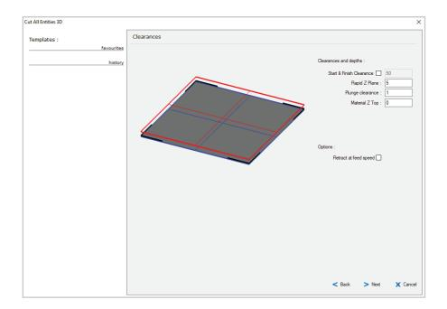
In the Clearances dialog, set Rapid Z Plane at 5 and Plunge Clearance to 1.
