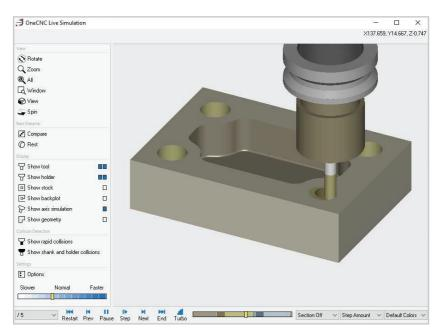
The Live Simulation window will open, and you can watch the toolpaths cutting away the material. The current coordinates of the tool are displayed in the top right corner.
