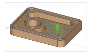
Toolpaths can be backplotted, which means they are drawn as geometry on a special layer named Backplot. Feed moves are drawn in green, and rapid moves in orange. Reposition moves in highspeed machining are drawn in blue.
