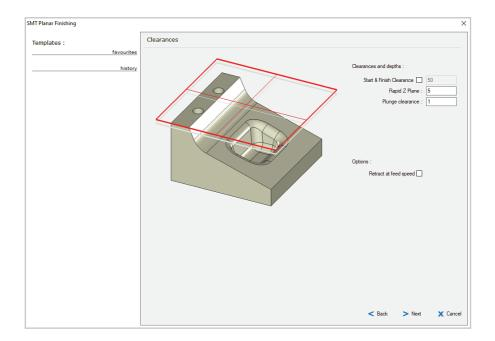
In the Clearances dialog, set the Rapid Z Plane at 5, and the Plunge clearance to 1.
