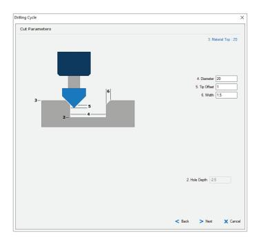
There are three settings in the Cut Parameters dialog for a Chamfer operation.
