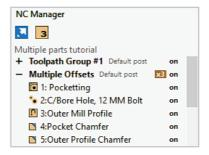
As we have only selected the work offsets for each repeat by their relative codes, which must be set on the machine itself, OneCNC has no information about the actual repeat position.
