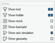
The Display options can be used to show or hide the tool, holder, stock, backplot, and geometry.
