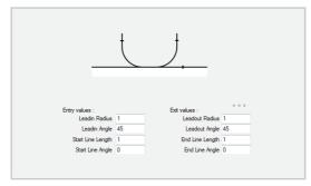
Start Line Length to 1 and set the Start Line Angle at 0. Copy the Entry values to the Exit values input boxes, and click Finished.
