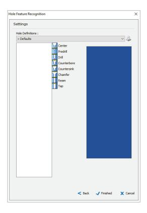
On the left of the Settings dialog is the Hole Operations list, where you can define multiple operations to apply to the selected holes.
