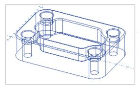
Turn off the Model and Geometry layers and you will see the extracted edges.
