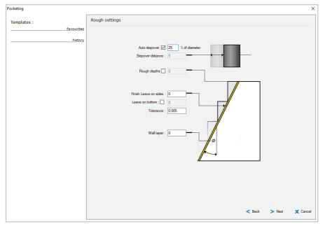
In the Rough settings dialog, stepover is the width of the cutting path. Select Auto stepover and set it to 25% of the tool diameter.
