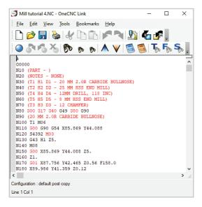
Specify the file location to save to, and the file will open in NC Link. The {TOOL\_SUMMARY} Tooling variable has inserted a list which shows the operator what tools are used and the station they are in.
