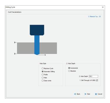
In the cut Parameters dialog there are a number of methods available to create the hole. Select Automatic drilling, which is the setting for OneCNC to create the drilling cycle.
