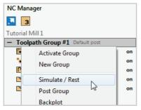
The NC Manager tab is shown at the right of the drawing window. Right click on the existing Toolpath Group #1, and select Simulate/Rest from the context menu.
