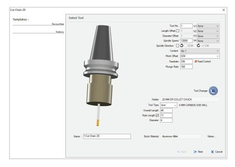
Select the 4mm carbide end mill tool from the Tool Library, and enter Tool No. 1. Set Coolant to No1 and Work Offset to G54. Select Aluminium Billet from the Material List, and click Next to continue.
