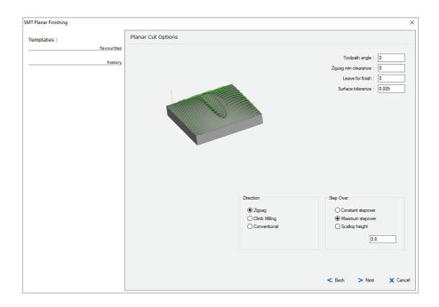
Set Direction to Zigzag, which allows the cutter to travel back and forth across the model. Single direction cut is possible, but this creates longer repositioning moves.
