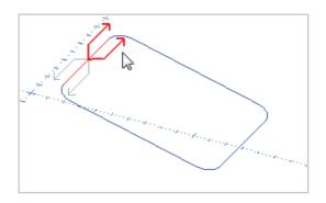
Pick the start point near the top of the chain, and click to set the direction of cut. It doesn't matter which side of the chain you are on as the center of the tool will travel on the geometry path.
