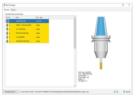
The Tool Changer dialog opens, with the Recent tab active. Tools you use regularly can be selected quickly from this tab.
