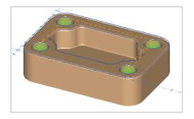
For a fixed display of the toolpath, right click on the Hole operation in the NC manager, and select Backplot from the context menu.
