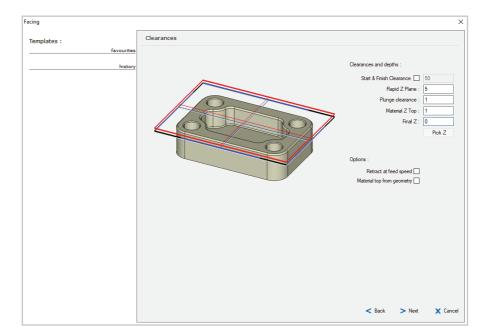
Start and Finish Clearance is shown as orange corners if enabled. It provides extra clearance before and after an operation. This is mainly used for multi-axis machining, while the part is repositioning.
