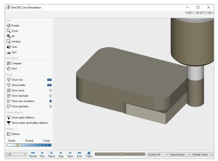
Simulate the new toolpath and you will see the cutter roughing and finishing the profile. When the cutter finishes the first roughing pass it will feed down and cut the second roughing pass. It will then retract before repositioning to begin the finish pass.
