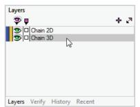
Turn off display of the Chain 2D layer, and select Chain 3D as the current layer.
