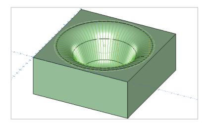
When you define a Radial toolpath you will be prompted for a center for the radial moves, which must be defined as a point entity.
