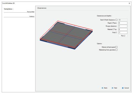
In the Clearances dialog, set Rapid Z Plane at 5 and Plunge Clearance to 1. Set Material top to 0 and Final Z at -1. Click Next to continue.
