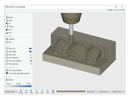
When used with a suitable tool, which must be able to end cut and remain centered, plunge roughing virtually eliminates lateral flexing of the cutter.
