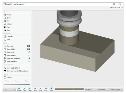
The simulation appears, showing the stock being faced back to the Z0 level.
