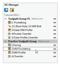
Before saving a template as a favorite, you should step through the toolpath wizard, checking the tool and settings used as you go, until you reach the last dialog in the wizard.
