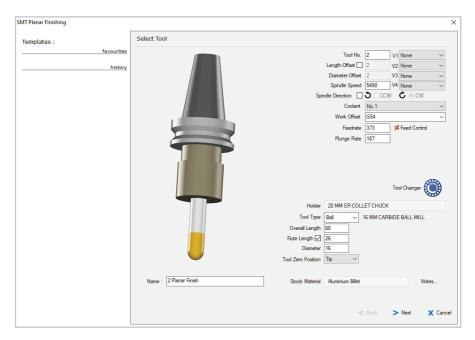
Select the 16mm carbide ball mill tool from the Tool Library. Enter Tool No. 2, and select Coolant No.1 and Work Offset G54. Select Aluminium Billet Stock.
