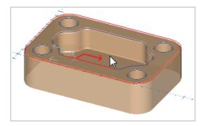
Click on a start position for the internal profile, and click as shown to set the side and direction. Press F3 to automatically select the complete profile.
