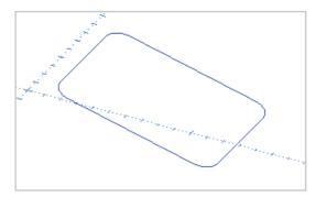
The display of the original chain has now been turned off, and the rotated copy is still visible on the new layer.
