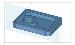
You can create a section view in the Views list using a plane positioned where you want the section.
