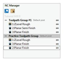
With the cursor over the new operation, hold down the left mouse button and move the operation up until a line appears between the Z Level Rough and Planar Finish operations.
