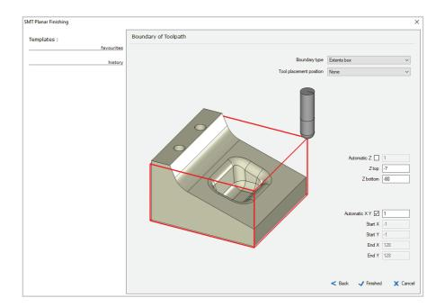
Select the Extents Box boundary type. Select None for tool placement, which allows the cutter centerline to travel up to the boundary.
