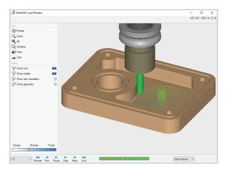
The Live Preview window shows an animated preview of the toolpath, backplotting as it goes. In Mill or Lathe the cutting tool will be shown traveling along the toolpath.
