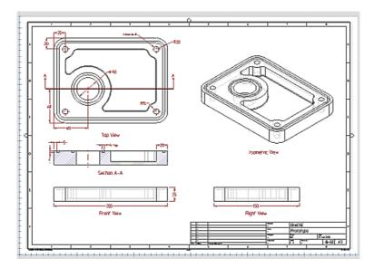
Traditionally, a technical drawing was the first step in production of a part. Now, you can design the part as a 3D model, and create one or more technical drawings automatically from the part.
