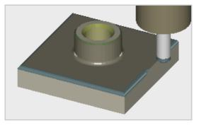
The Corner Rounding toolpath is specifically designed for the application of corner rounding tools to an edge of a part. It is applied to a selected chain, and is similar to the chamfer operation as the Z level of the toolpath is set relative to the selected geometry chain.
