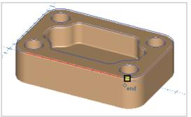
Select the last entity in the profile to cut, or press F3 to automatically select to the end of the chain.
