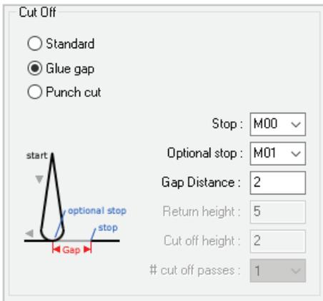
In the Cut Off section of the 4 axis wire cut dialog, select the Glue gap option.
