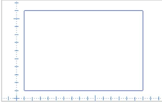
Enter coordinates in the toolbox or use a grid snap to start the rectangle at X10 Y10. You can then enter 150 for Length and 100 for Height to make the rectangle 150 wide in X and 100 high in Y.
